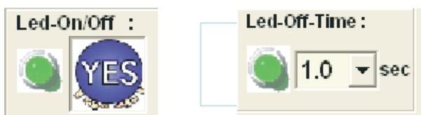
a. "YES". During normal operation, Led is green. LED is red when it is alarm or error. e.g.(When power is not enough, red is flash)
