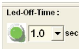
2-31. "LED-Off Time" Can be set from 0~4seconds.Short time means more power consumption. LED on time is always 0.4 second. When you choose 1 second, then LED on is for 0.4 second, LED off is for 1 second. On and off is cycled.
